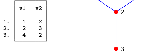
Example of an edge list and its corresponding graph (undirected and unweighted). Drawn using NETPLOT (Corten, 2011).
