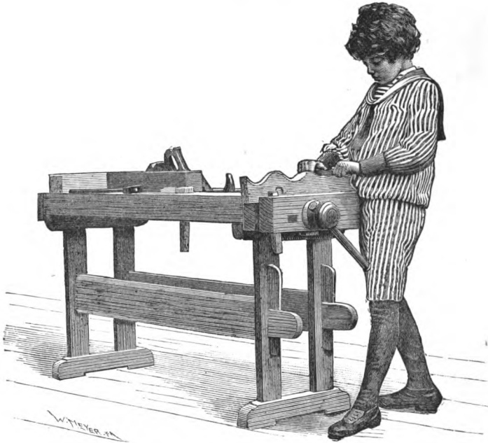
Plate VIII. Position: Smoothing, &c., with the spokeshave.
