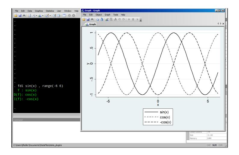
Sympy can also be used to find the functional form of derivatives and integrals. Here is a command for graphing a function with its derivative and integral.
