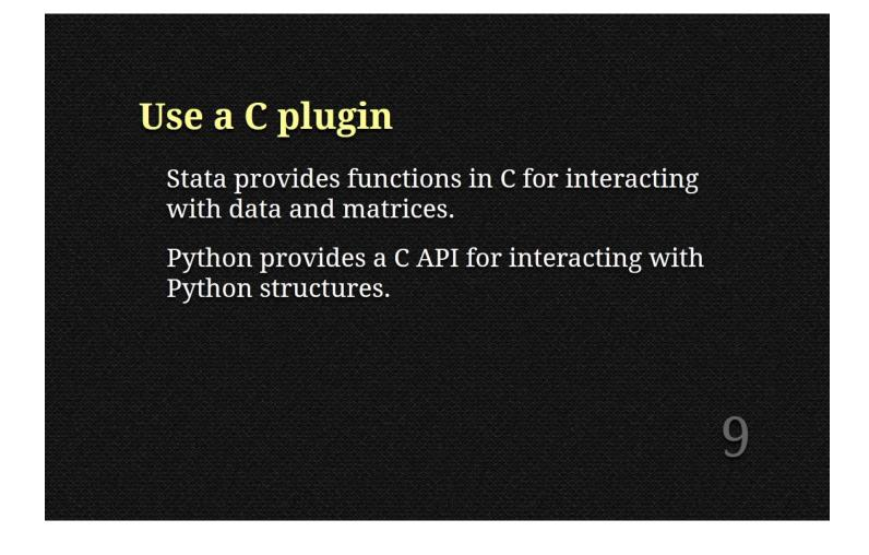
Stata, through its plugin system, provides C functions for interacting with Stata data, macros, matrices, etc. Python, through its C API (application programming interface) provides C functions for starting a Python interpreter and interacting with Python structures.
